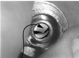
Section of ceramic sleeve broken out within the connector
